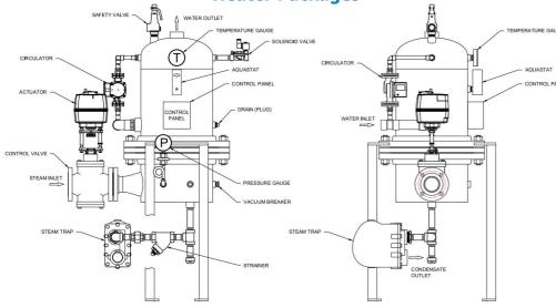
Each ALSTROM Units are equipped with universal, microprocessor based single point temperature controller including Modbus communication. Clear LED readout, it is designed to handle fast control loops with fluctuating loads, permitting precise temperature regulation.
